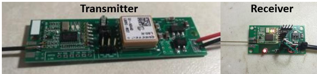
Figure 3-58. Eggfinder GPS Tracking Device
