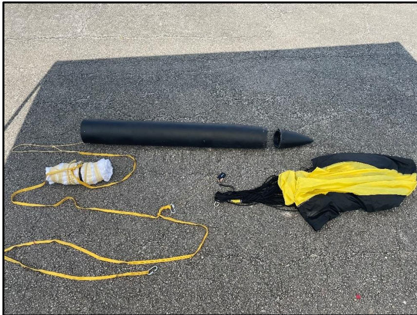
Figure 5-4. Upper Payload Bay Sustained Damage
