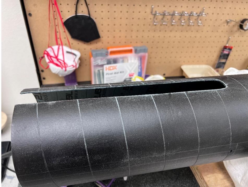
Figure 3-44. Old Fin Slots on Airframe
